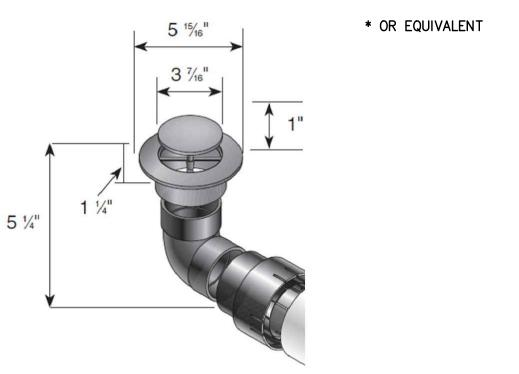
Part #: 430 Material: High Density Polypropylene (HDPE) Load Recommendation Guide Colors: Green Fits: 3" and 4" corrugated, sewer, triple wall pipe and 4" Sch. 40 pipe Class A Open Surface Area: 10 Sq. Inches Loads of 1-60 psi. Spring: Stainless Steel Grade 302 Recommended for pedestrians, bicycles and wheel Open Pressure: 0.04 PSI
