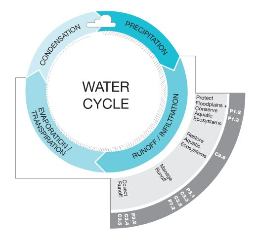
This diagram illustrates how prerequisites and credits in the SITES v2 Rating System relate to and support the processes of the natural water cycle, shown highlighted in the blue circle above. The bottom right shows the actions that SITES encourages in gray, while the corresponding prerequisite and credit numbers are shown in the dark gray bar.
